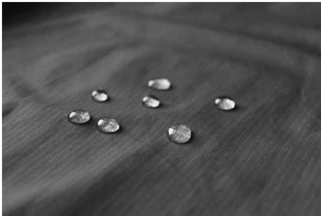
Figure 9.2 Effect of a durable water repellent (DWR) finish applied to a fabric surface on the contact angle of water.
